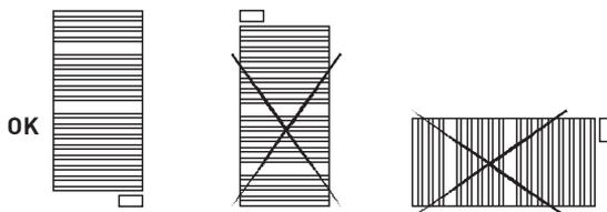
**IMPORTANT** - This product must never be installed with its control panel at the top. This product must not be installed horizontally. During installation, use wedges so that the control panel will not be in contact with the floor.
