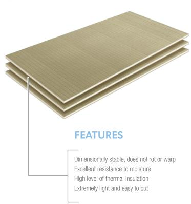
The thermal panel is a lightweight insulated tile backing board developed specifically for use with tile floors. It consists of a polyfoam core with glass fibre reinforced polymer-modified cement faces, making it the ideal substrate for floor tiling and under tile heating systems.
